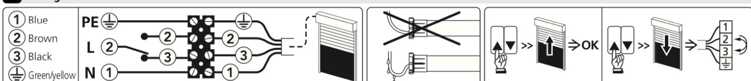
**⚠ - 3 operators (max.) can be wired in parallel on one switch.**
